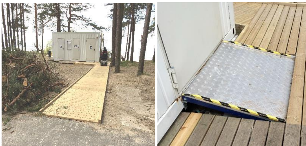
Figure 23. New beach road to the outdoor toilet in Pirita and an inaccessible disabled toilet (ascending ramp and a dangerous edge)
