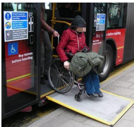
Figure 6. A low-floor bus with an automatic ramp in London
